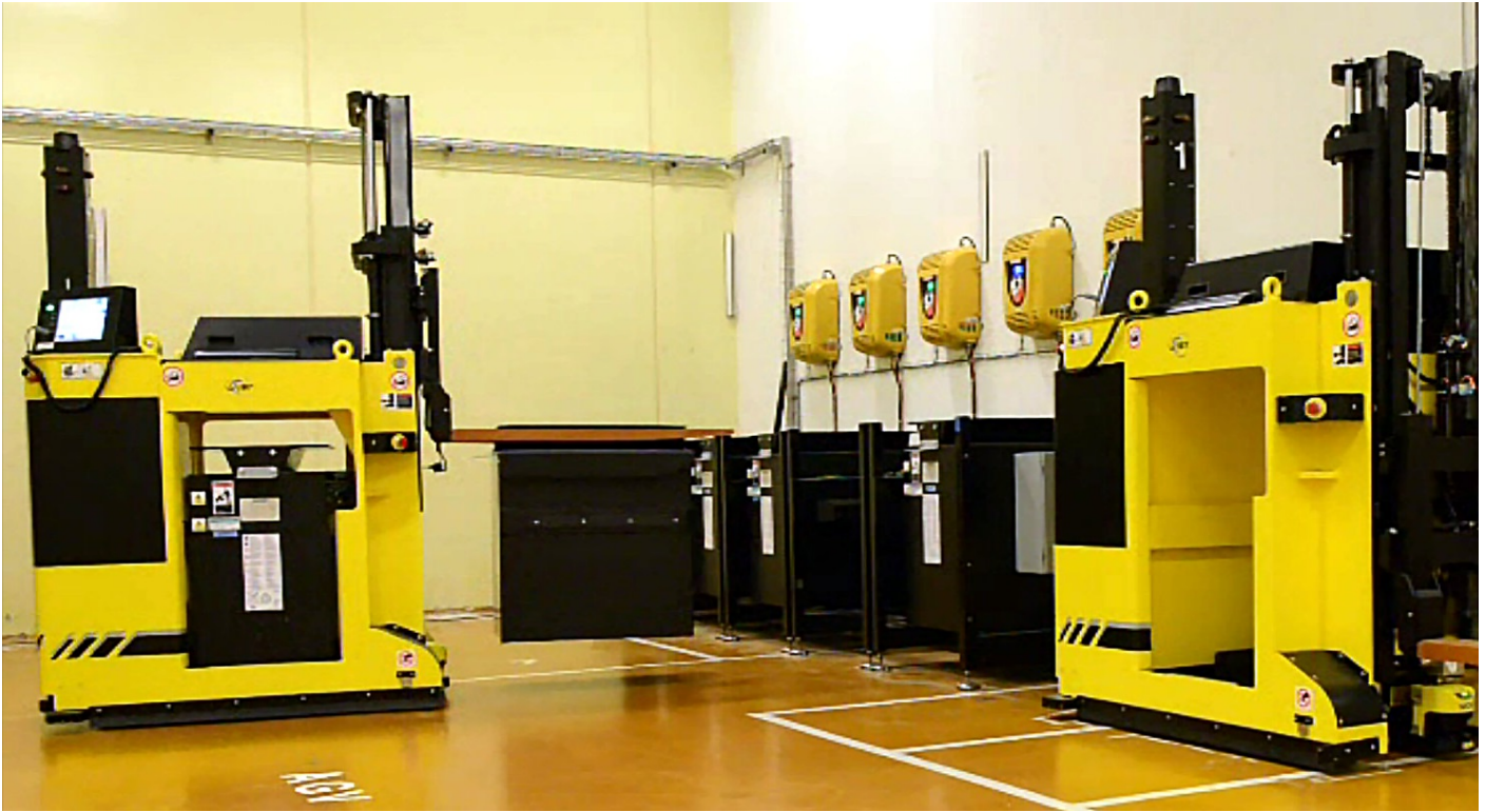
SGVs automatically exchange batteries during operation
