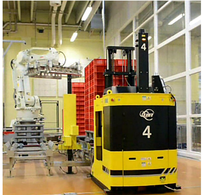
SGV automatically picks up a pallet of full trays from one of two robotic filling lines
