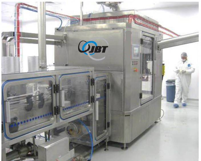
▲ JBT SeamTec™ Pre-gassing Closer with gas-tight guarding
