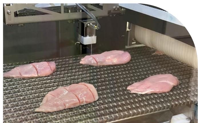
These can be strips, splits, steaks or dices. Multiple products can be cut using the same slicer configuration. Cutting blades at fixed or adjustable widths give you flexibility.
