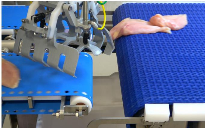
*Overlapping products will automatically be rejected, preventing them from cluttering the production.*
