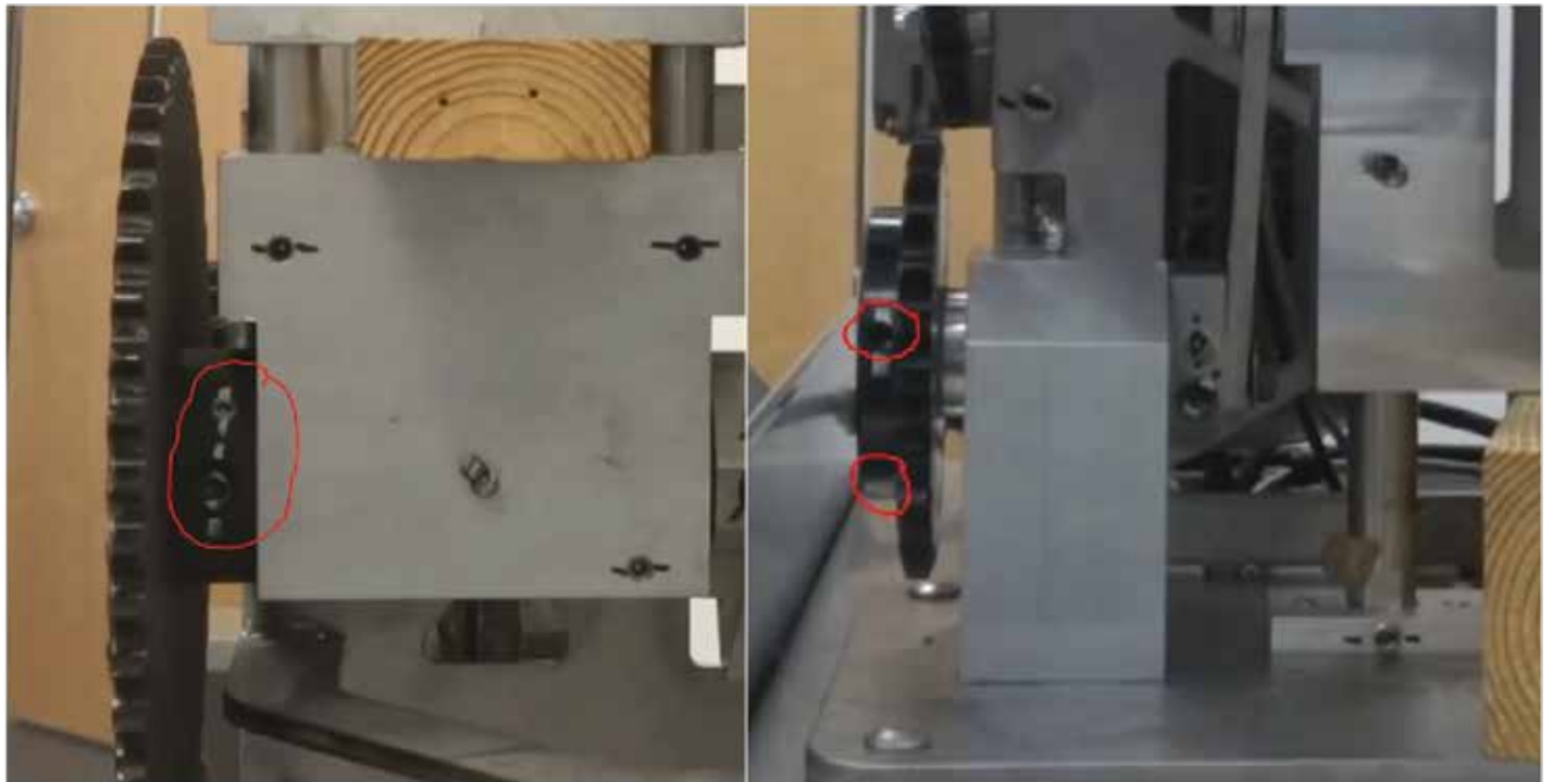
Figure 16. Loosen Set Screws and Socket Head Screws and Remove Sprockets and Shafts
