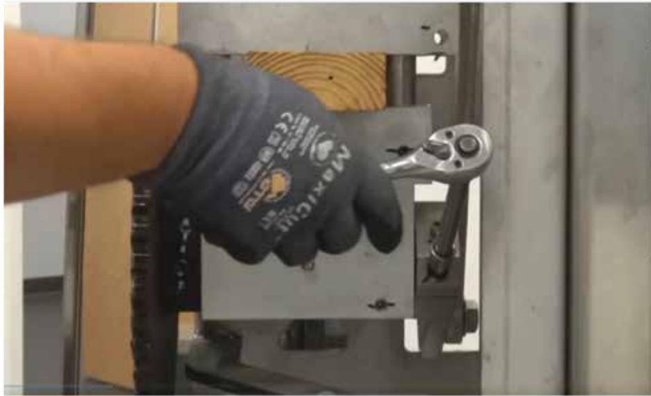
Figure 12. Use Allen Wrench to Loosen Upper Cup Crank Arm.
