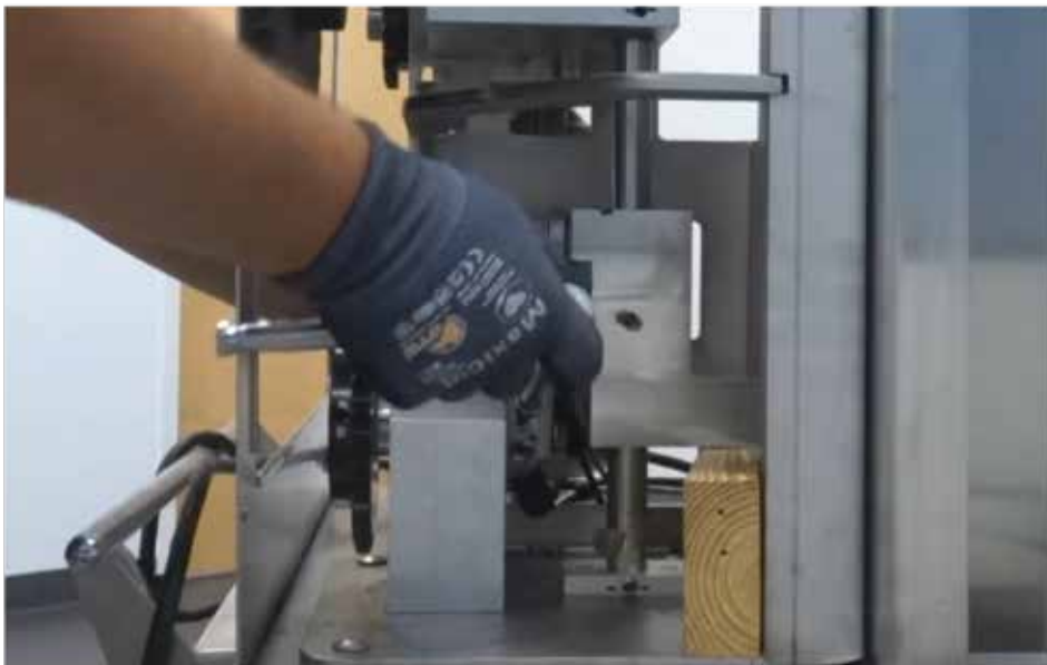
Figure 13. Loosening Lower Crank Arm.
