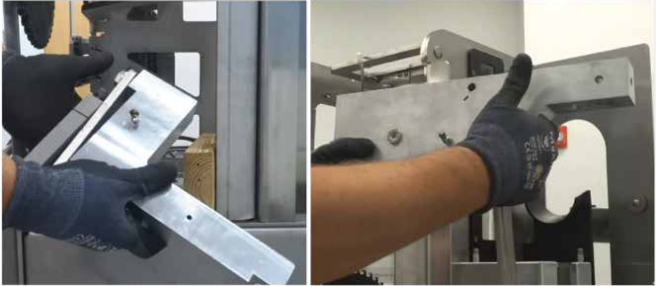
Figure 15. Removal of Upper and Lower Drive Arms with Linkages and Crank Arms
