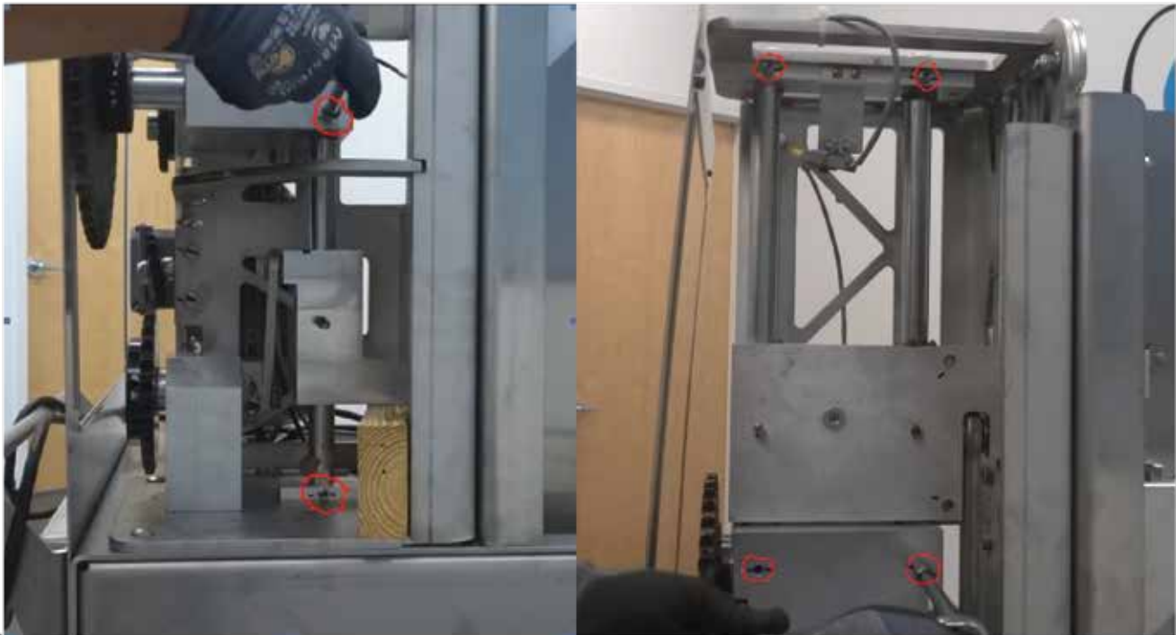
Figure 14. Removal of Linear Shafts
